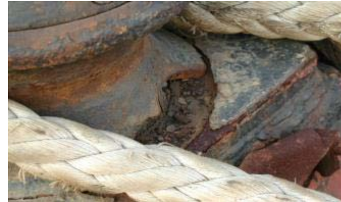
Tow line fairlead condition 拖缆导缆鐘
